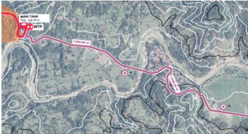
Figure 9 - Loihuno Transmission Main. Pressure Break Tanks
