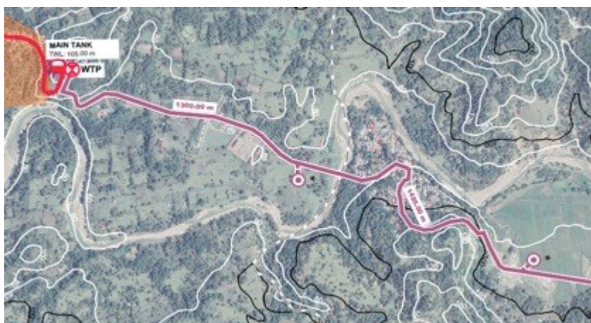
Figure 4-9 - Loihuno Transmission Main. Pressure Break Tanks
